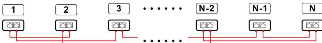
**Note:** Max of 12 units. The best practice is to minimize the number of jumps between inverters by alternating between 1 and 2 jumps on each inverter.
